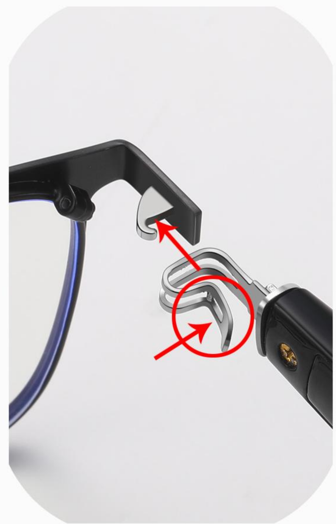
第四步 STEP 4 : 按压红圈部分, 按箭头 方向插入使卡扣扣住, 完成换腿组装 Press like STEP 1, push in the snap-fit, after hooked, assembly successfully
